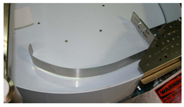
The new Feed Guide for the Model 793 slicer is retrofitable to all Model 793 slicers.
